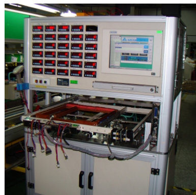
Auto Test Machine: Function, Waveform, Inrush Current, LED, Fan Speed Detector, Others
